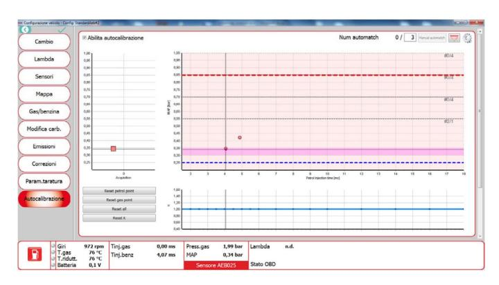
Step one can be concluded as soon as the red line is plotted, but optionally the driver can refine the acquisition continuing the petrol drive.
