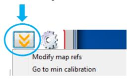
Modify map refs: opens a setup window for the calibration of the references of the map, and the admitted range of the K.
