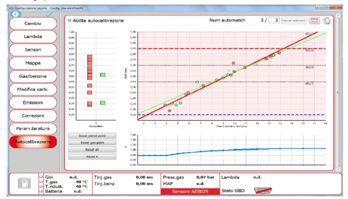
• **Red rhombus dot**: is the current working point of the acquisition. It is visible only if the ECU is connected and the engine is on, and the fuel is petrol. Around rhombus there is a highlighted line dark red, show you the subzone of the zone where you drive. You can collect one point for each subzone, there are 4 subzone for each one of them.
